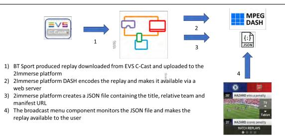
Figure 18: Replay capture, encoding and delivery workflow
