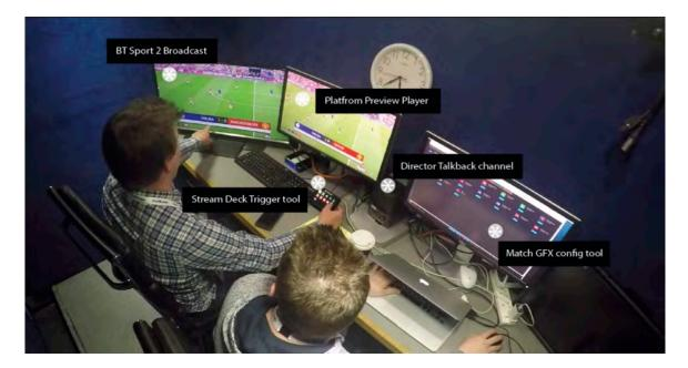
Figure 4: The setup of the system in the OB truck at the stadium
