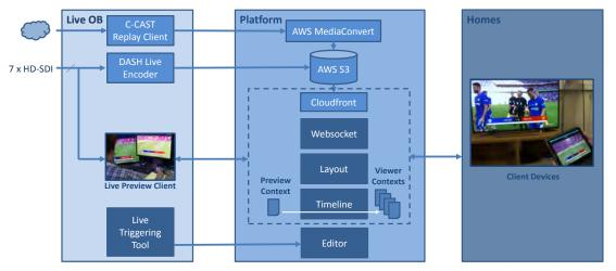
Figure 17. 2-IMMERSE Platform services used during the end-to-end live tests
