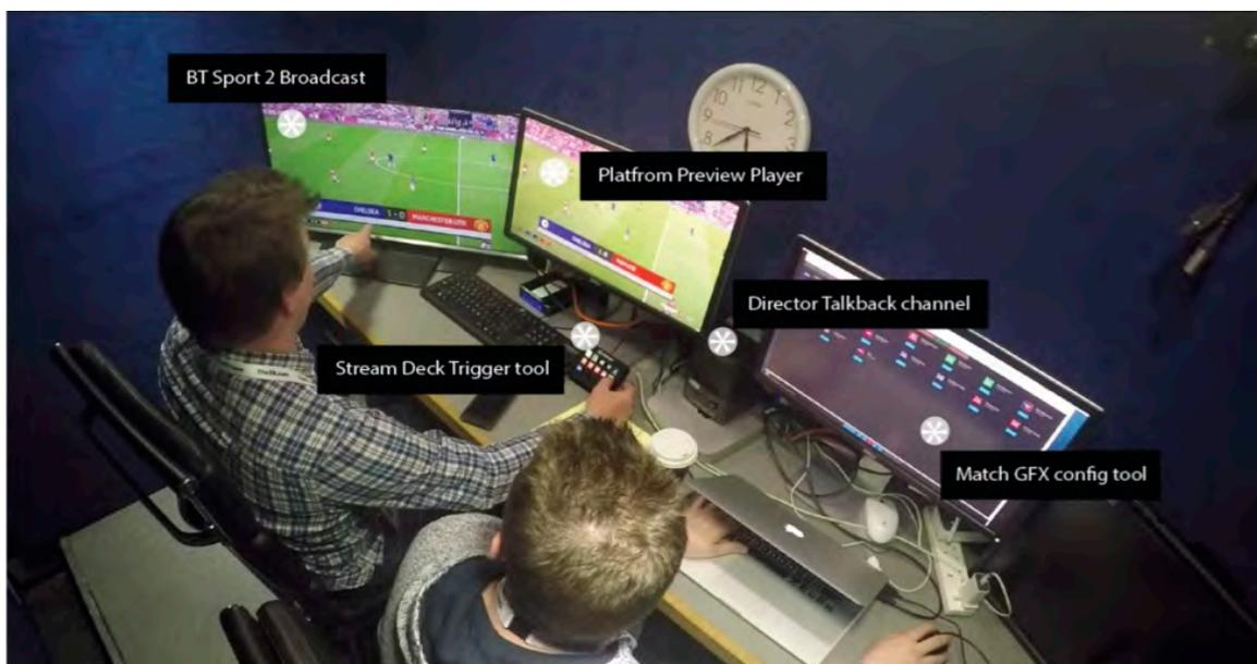
**Figure 4: The setup of the system in the OB truck at the stadium**
