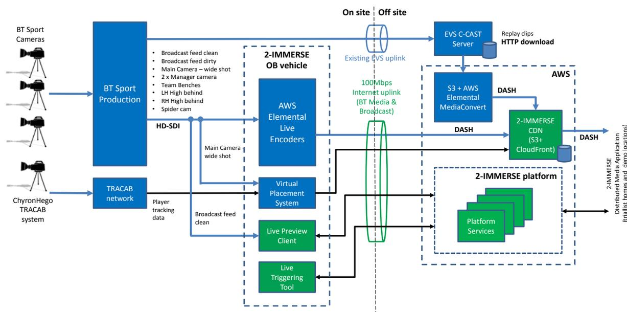
Figure 16. System architecture for 2-IMMERSE live end-to-end tests.
