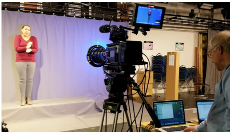
Figure 87 Capturing the interpreter using blue LED lights and Chromatte (reflective cloth) at BBC R&D.
