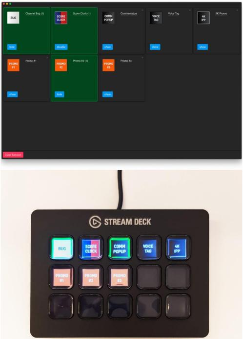
Figure 51 The live triggering tool (top) and hardware device StreamDeck (bottom) triggering launcher.
