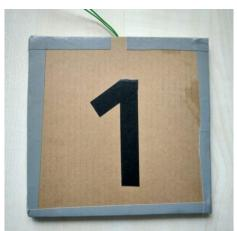
Figure 70 Prototype of a floor pad sensor build from carton, aluminium foil and adhesive tape
