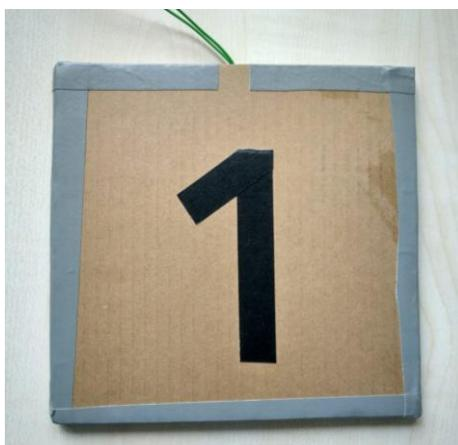
**Figure 70 Prototype of a floor pad sensor built from carton, aluminium foil and adhesive tape**
