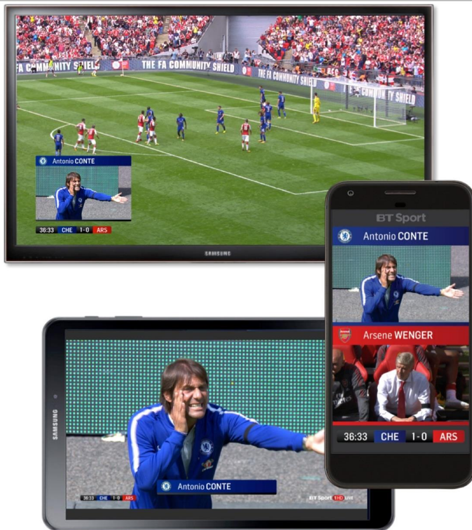
Figure 21 A multi-screen compilation of the Manager Cam layout options across 3 screens. The viewer has the option of selecting manager cam feeds for one or both teams to supplement the live match action. Note the flexible rendering of the GFX (manager name) as an overlay or as a BT Box title depending on video render size.
