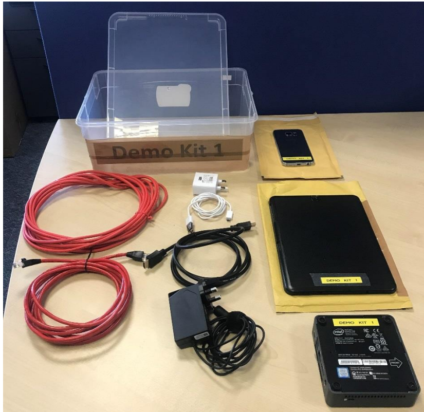
Figure 19 A trial kit (one of eight kits) showing the small computer, tablet, phone and cables.
