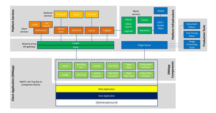
Figure 1: 2-IMMERSE Platform Architecture for the First Release
